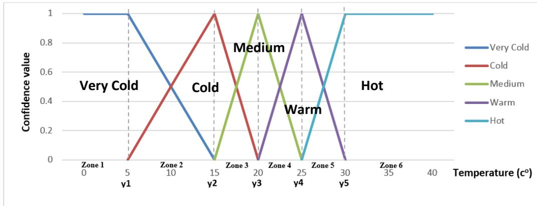
Figure 6: Membership function graph of weather temperature
