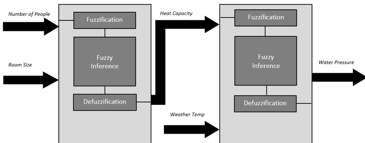
Figure 2: Fuzzy Logic Controller of Roof Sprinkler Cooling System
